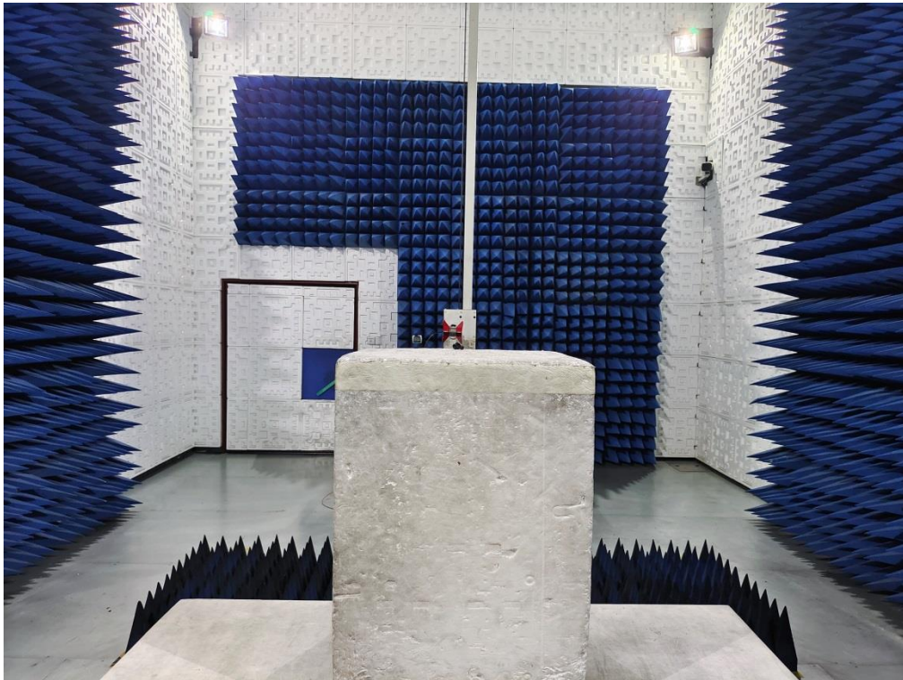
RADIATED EMISSION TEST SETUP ABOVE 1GHz
