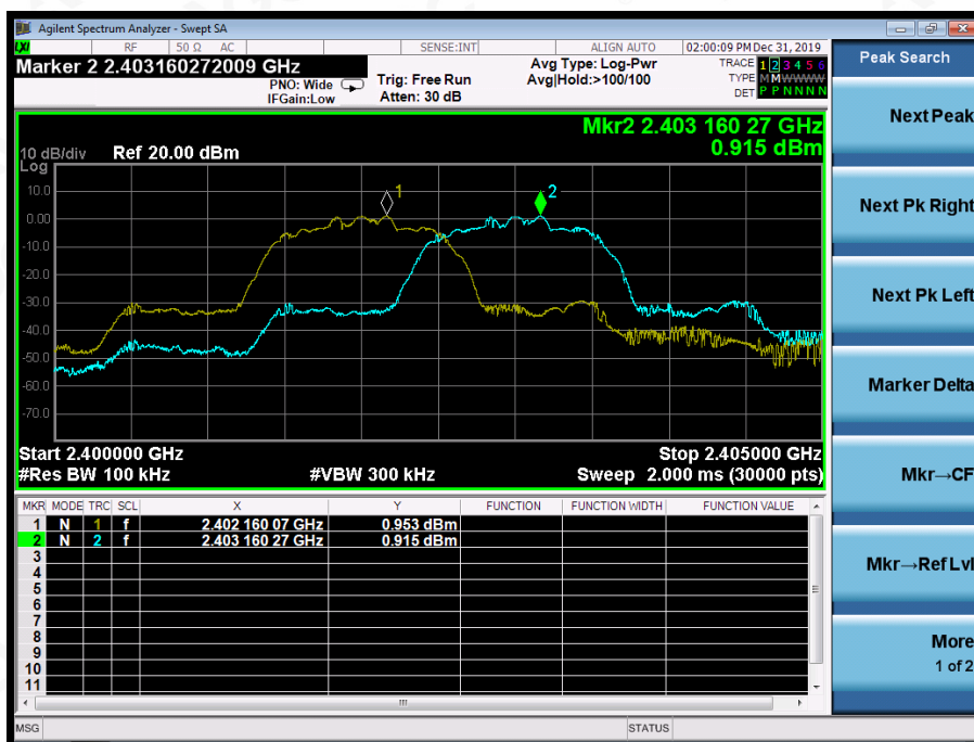
TEST PLOT FOR FREQUENCY SEPARATION
