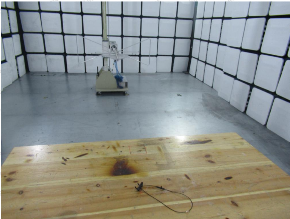
Photo of Radiation Emission Test
