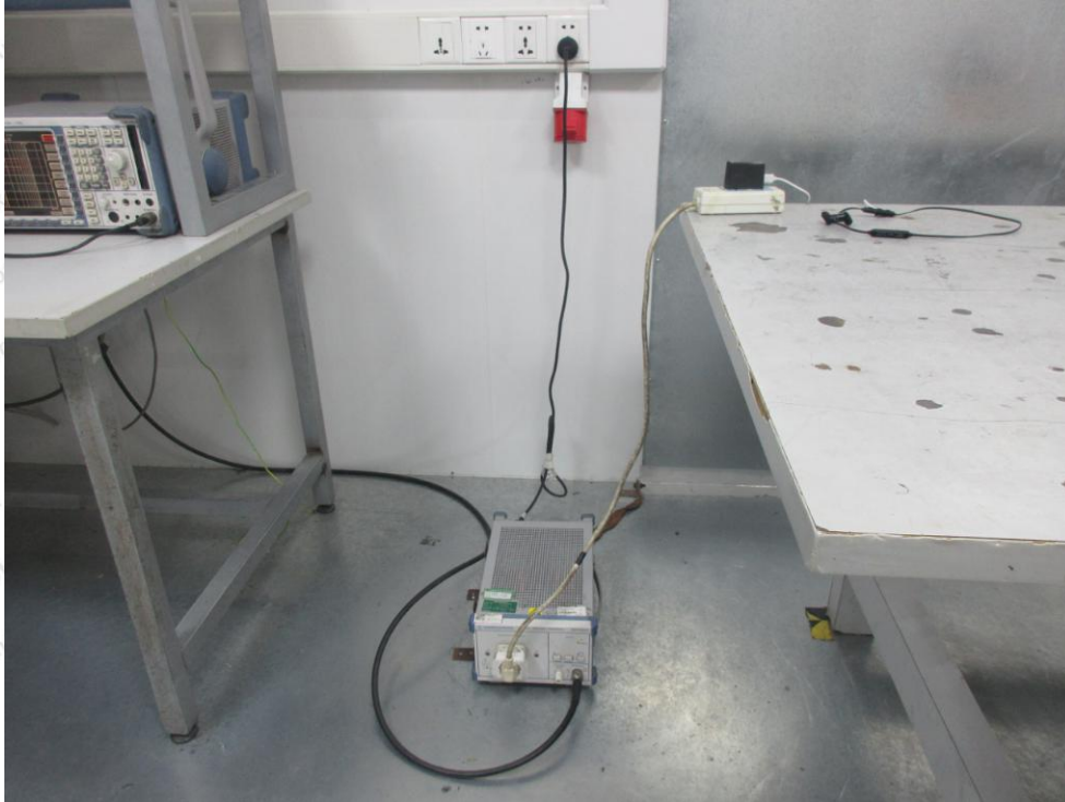
Photo of Conducted Emission Measurement
