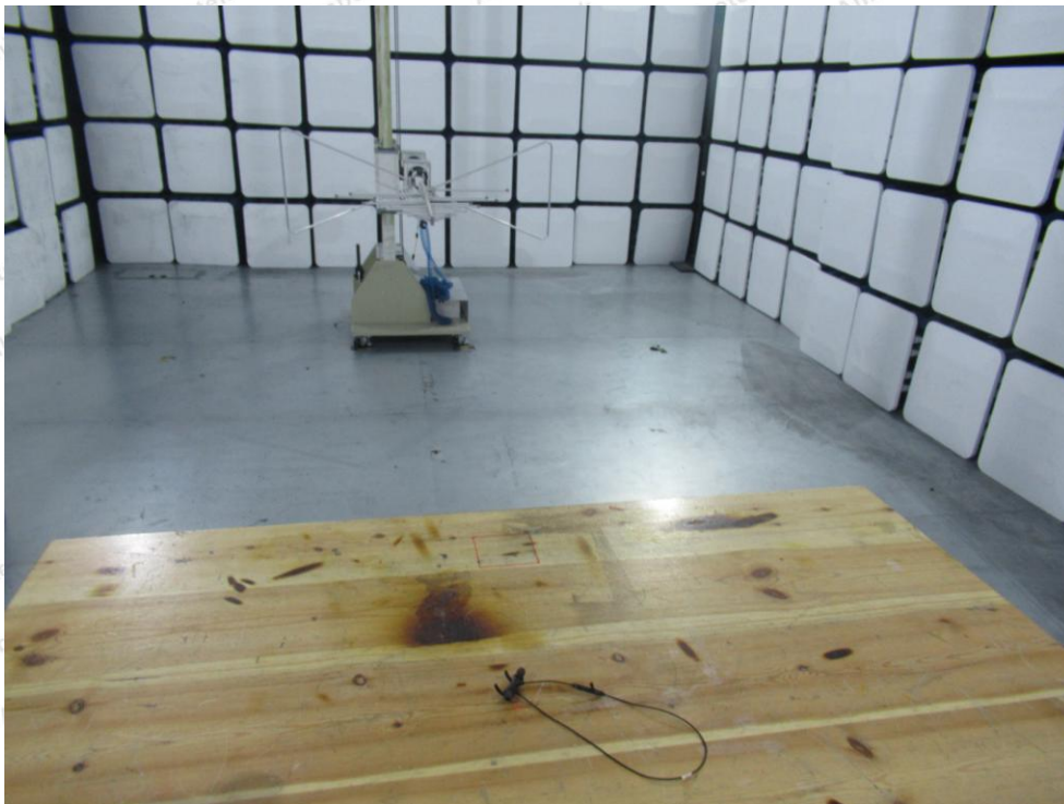
Photo of Radiation Emission Test
