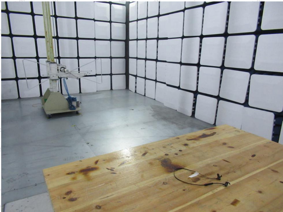
Photo of Radiation Emission Test
