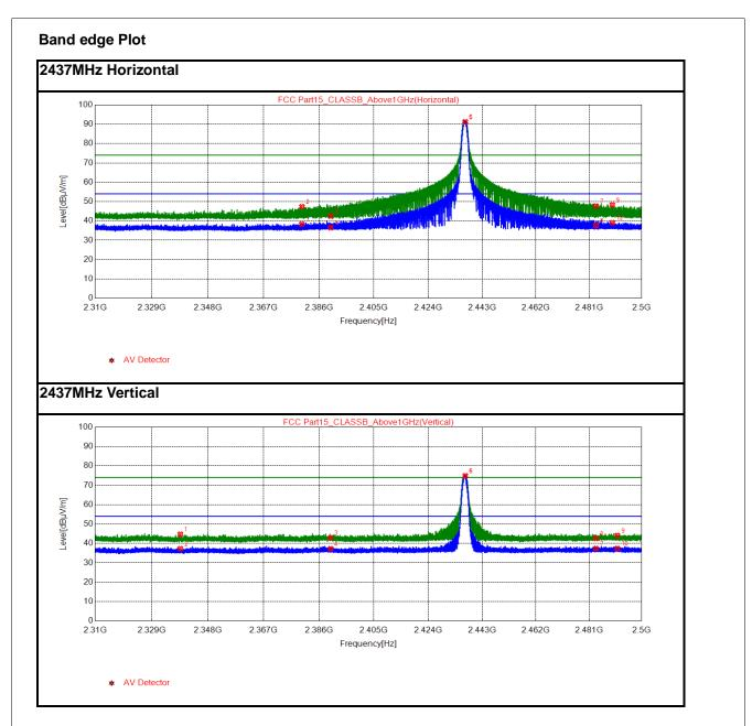
Note: The green line is the PK detection method and The red line is the AV detection method.
