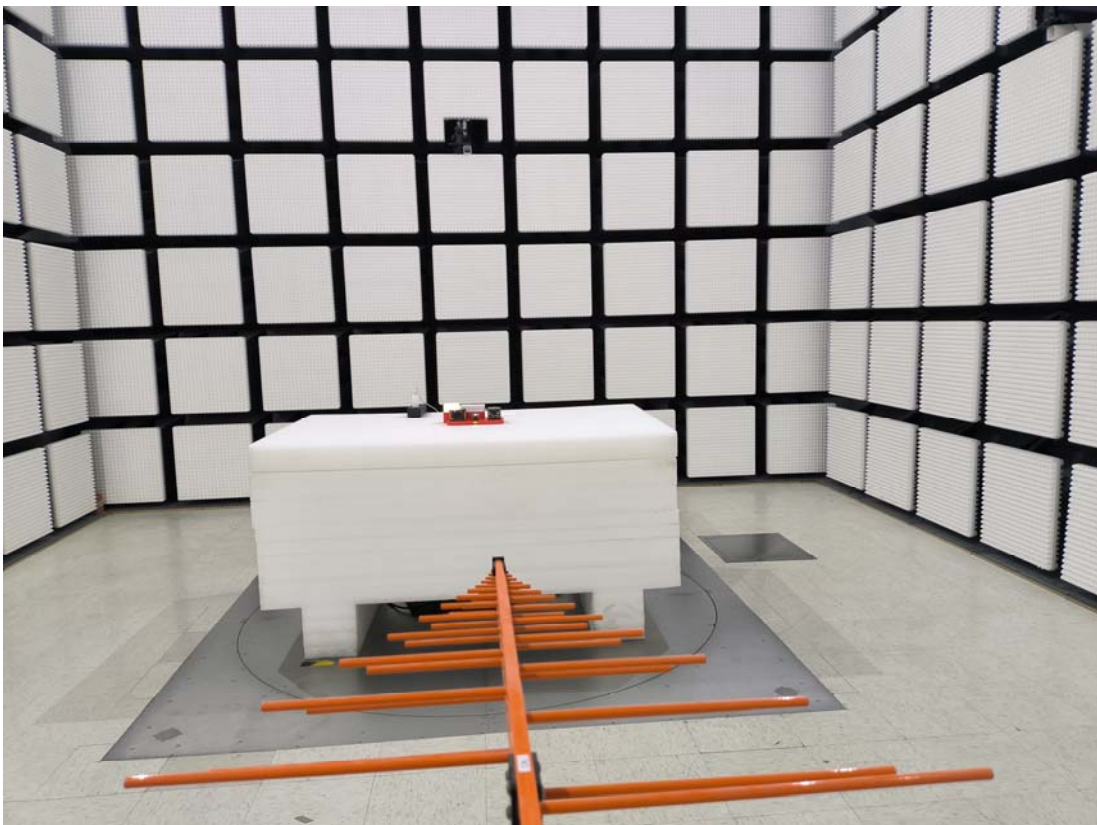
Radiated Emission 30M-1GHz View
