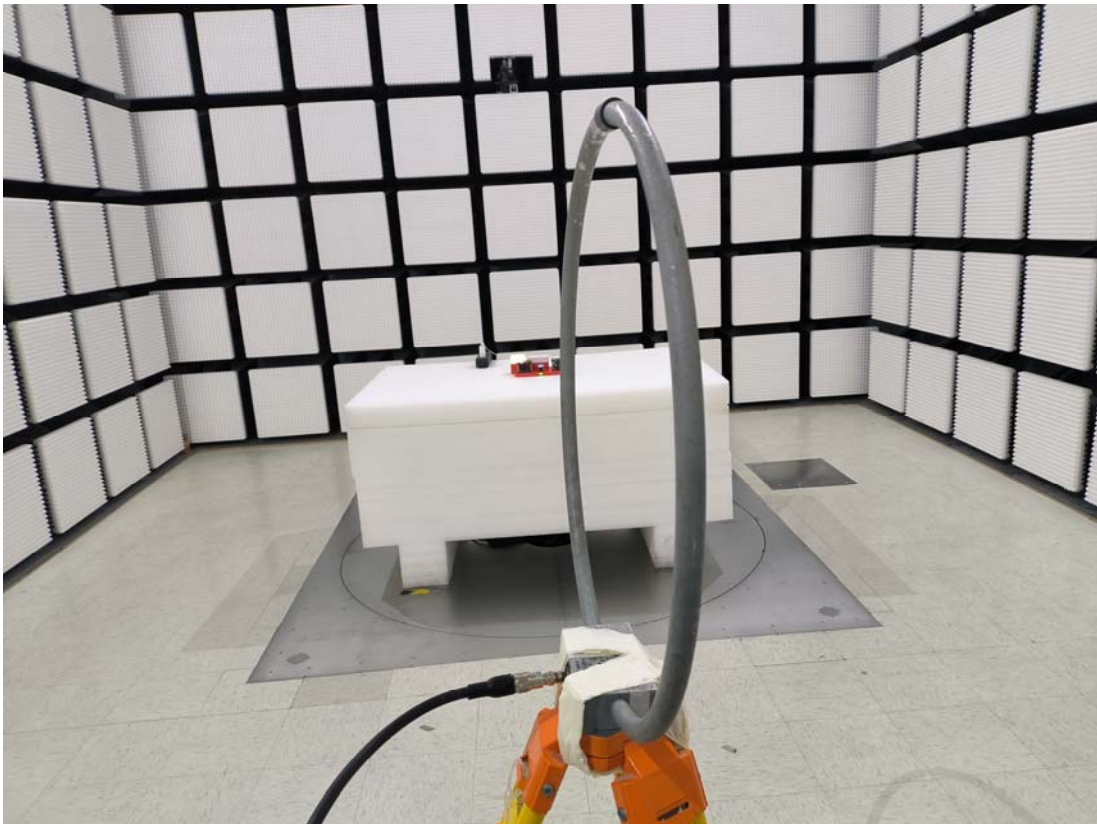
Radiated Emission 9k-30MHz Perpendicular View
