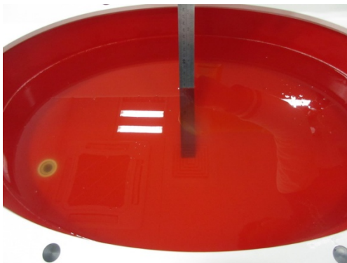
Liquid depth in the flat Phantom ( \geq 15\text{cm} depth) HSL(750MHz)
