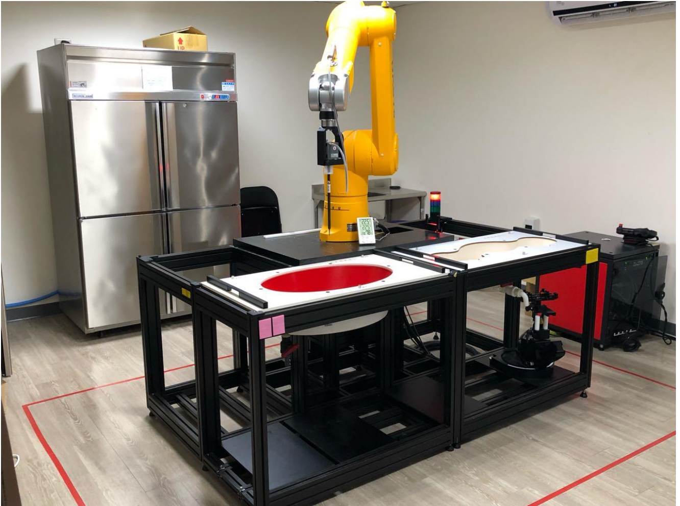
Liquid depth in the flat Phantom ( \geq 15\text{cm} depth) HSL(750MHz) HSL (1750-3800MHz)
