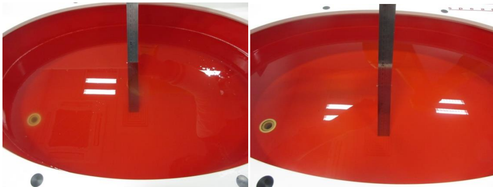
Liquid depth in the flat Phantom ( \geq 15\text{cm} depth) HSL(750MHz) HSL (1750-3800MHz)
