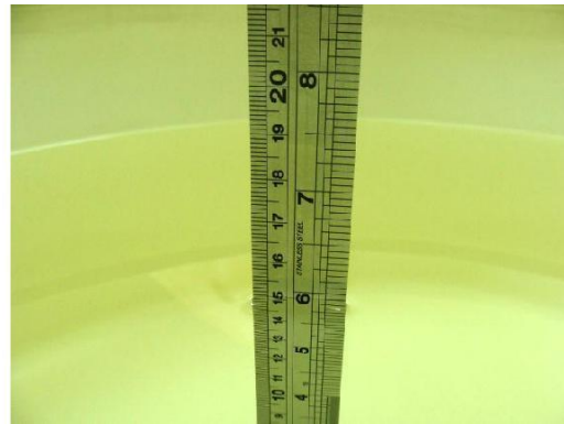
Fig 5.2 Photo of Liquid Height for Body SAR
