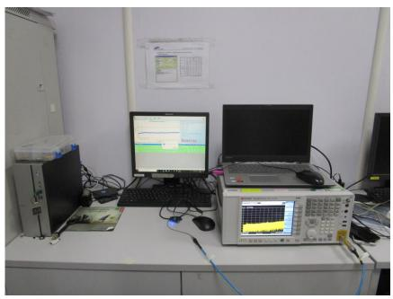
1.2 Conducted Emissions at AC Power Line (150kHz-30MHz) Test Setup
