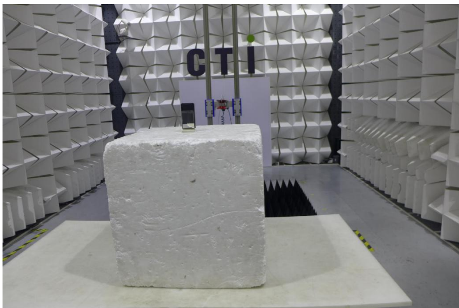
Radiated spurious emission Test Setup-3(Above 1GHz)
