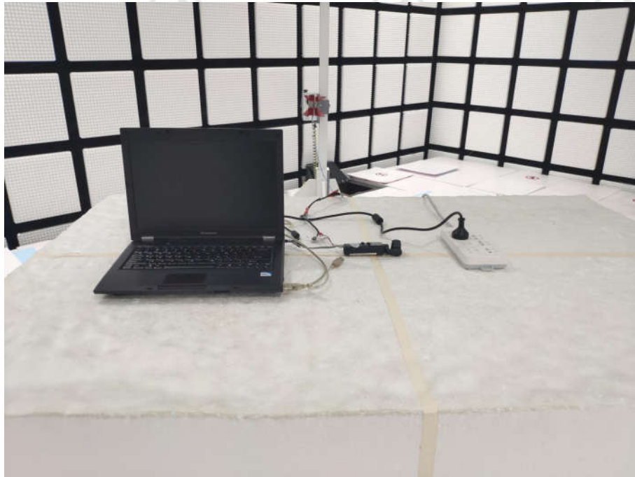
Radiated spurious emission Test Setup-3(Above 1GHz)
