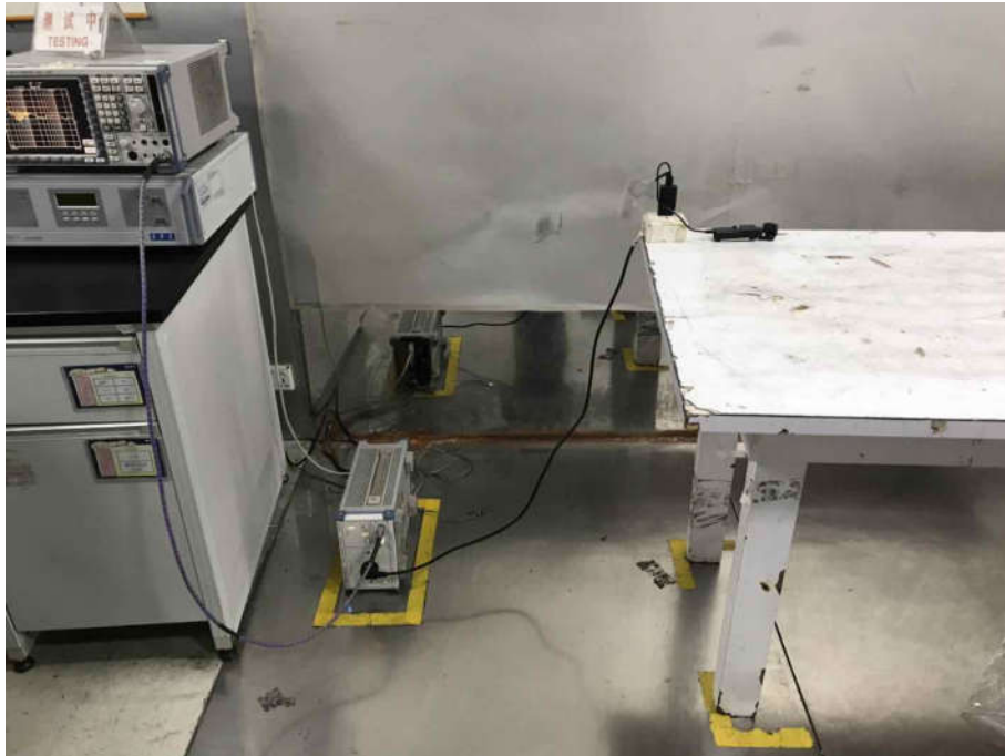
Conducted Emissions Test Setup
