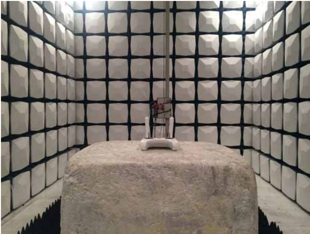
Description: Radiated Emission Test Setup for 1~18GHz
