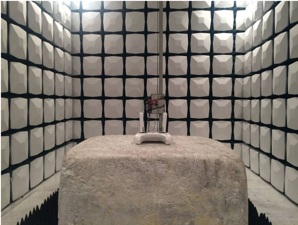
Description: Radiated Emission Test Setup for 1~18GHz
