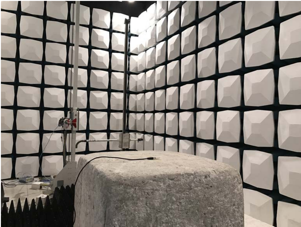
Description: Radiated Emission Test Setup for 1~18GHz
