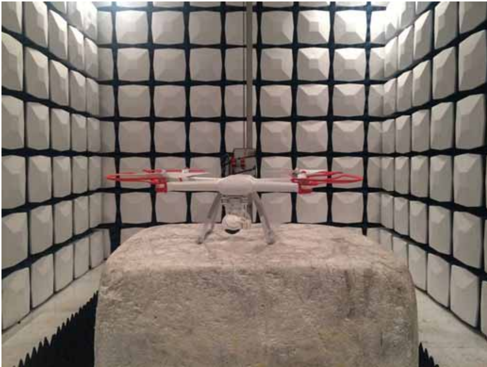
Description: Radiated Emission Test Setup for 1~18GHz
