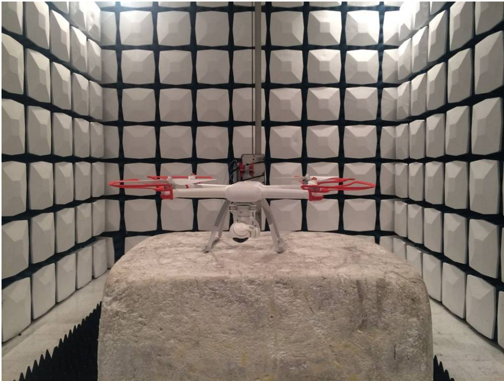
Description: Radiated Emission Test Setup for 1~18GHz
