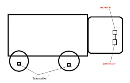
VR-308B series include three parts of transmitter, repeater and projector. Internal projector and external projector are two ways to fix projector to satisfy different needs. Internal projector is standard configration, we provide two types for you to choose, binding and valve.
