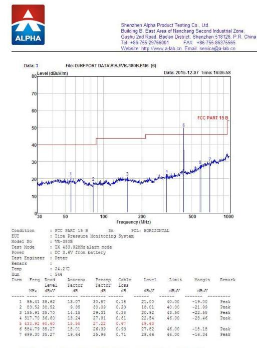
Remark: Level = Read Level + Antenna Factor - Preamp Factor + Cable Loss
