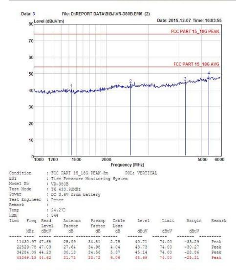
Remark: Level = Read Level + Antenna Factor - Preamp Factor + Cable Loss
