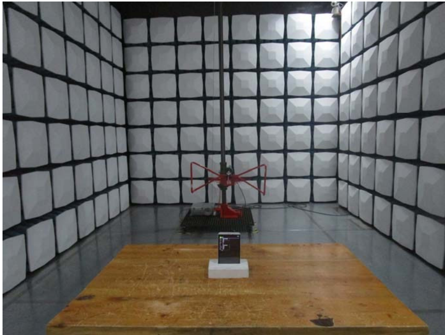
Radiated Emission View (Below 1GHz)
