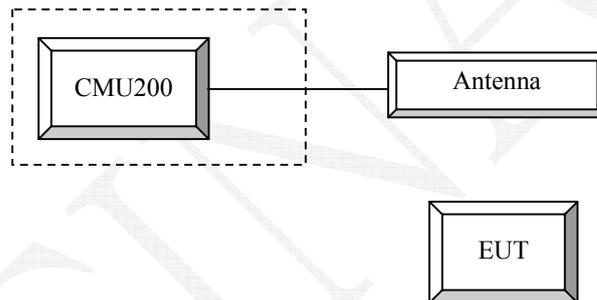
**Block Diagram of Test Setup**
