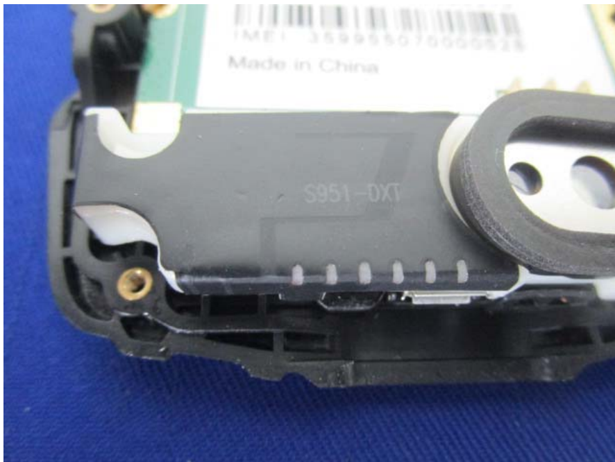
EUT – GSM&WCDMA Antenna View
