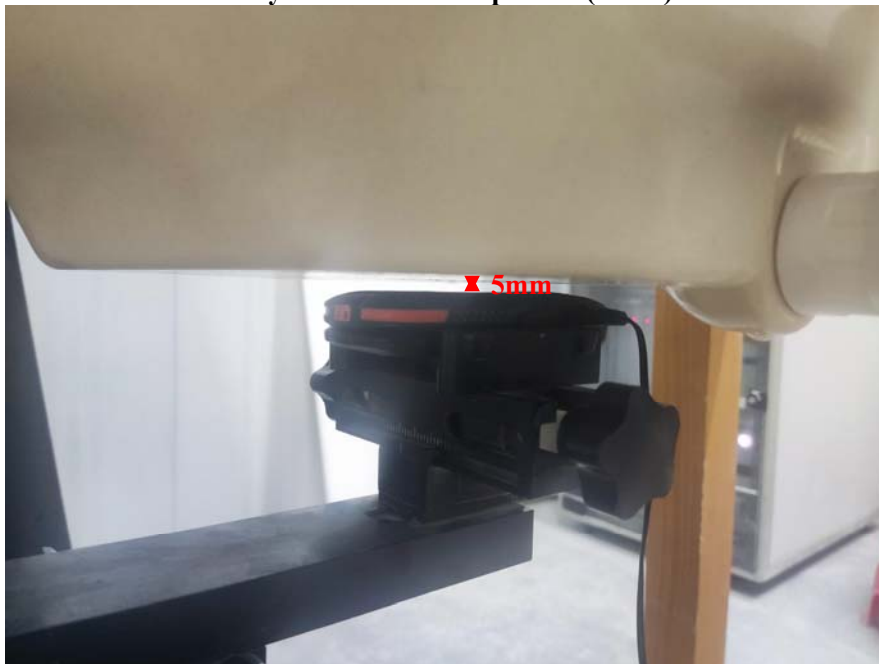
Body Worn Back Setup Photo(5 mm)
