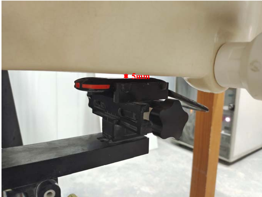
Body Worn Back Setup Photo(5 mm)
