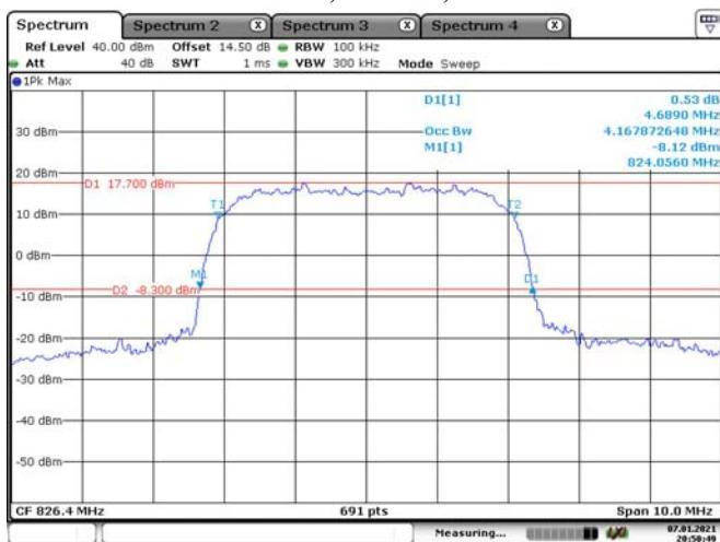
**WCDMA Band V, HSUPA, Middle Channel**
