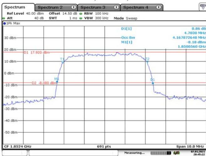
**WCDMA Band II, HSUPA, Middle Channel**
