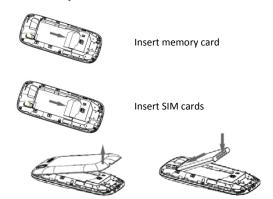
Install battery and battery cover
