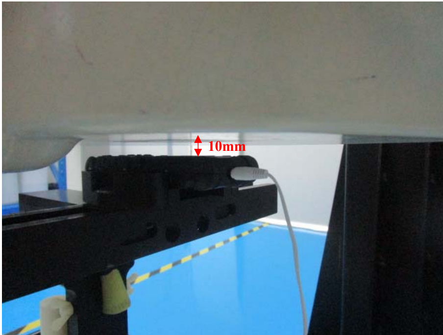
Body-worn Headset Setup Photo
