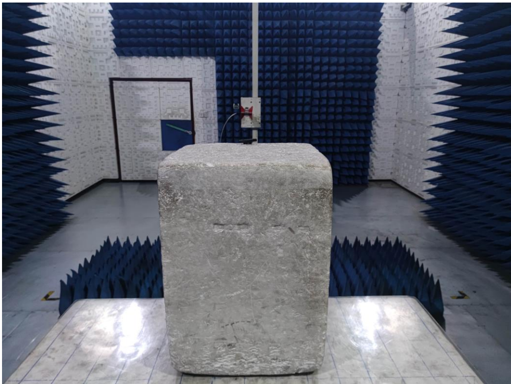
RADIATED EMISSION TEST SETUP ABOVE 1GHz
