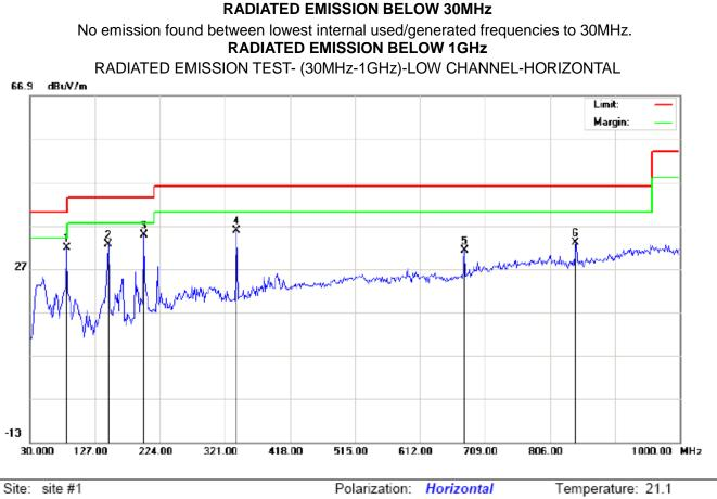
Limit: FCC Class B 3M Radiation EUT: WiSe 1230 BLE Module M/N: WiSe1230 Mode: Low Channel TX Note:
