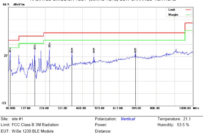
RADIATED EMISSION TEST- (30MHz-1GHz)-LOW CHANNEL -VERTICAL
