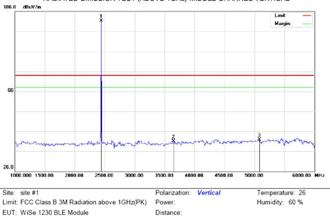
RADIATED EMISSION TEST-(ABOVE 1GHz)-MIDDLE CHANNEL-VERTICAL
