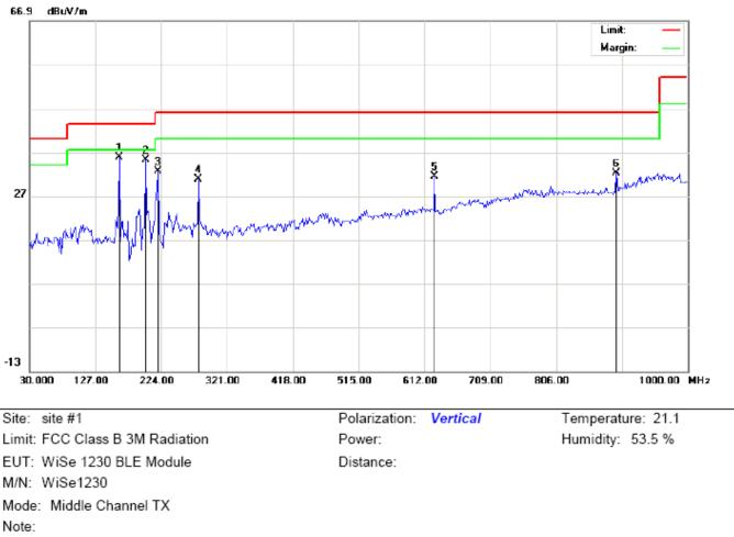
RADIATED EMISSION TEST- (30MHz-1GHz)- MIDDLE CHANNEL -VERTICAL
