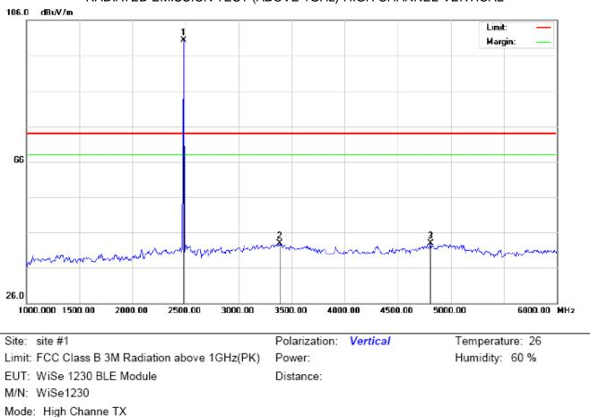
RADIATED EMISSION TEST-(ABOVE 1GHz)-HIGH CHANNEL-VERTICAL
