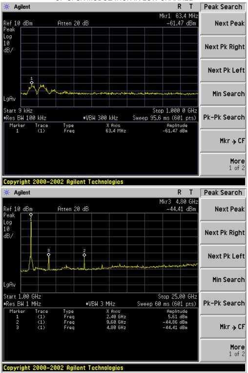
TEST PLOT OF OUT OF BAND EMISSIONS WITH THE WORST CASE OF GFSK MODULATION IN LOW CHANNEL
