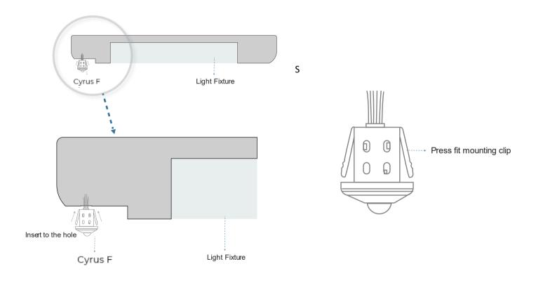
The press fit mounting clip on the device will keep it attached to the fixture
