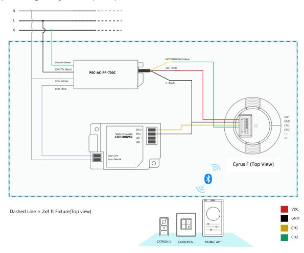
Set the output channel mode of the Cyrus F as 'single channel' in the mobile application
