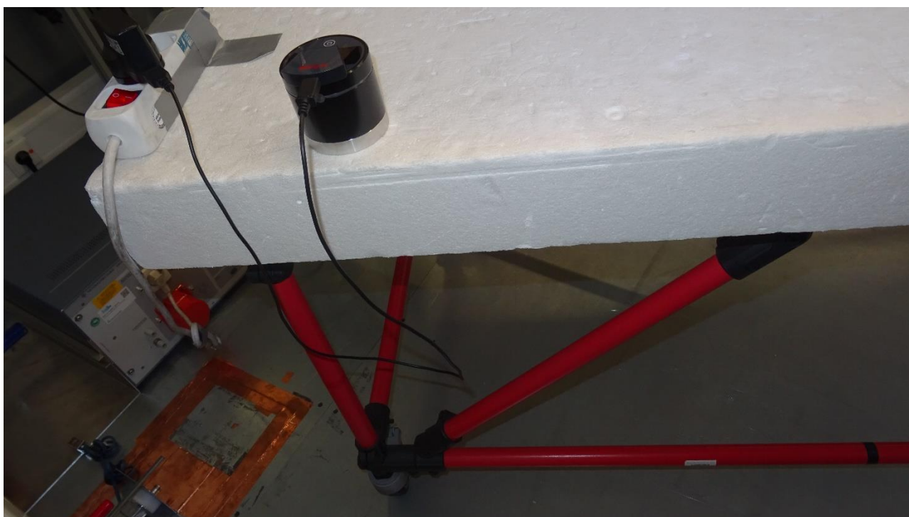
Picture 12: Test setup AC power line conducted emissions (rear view), charging mode
