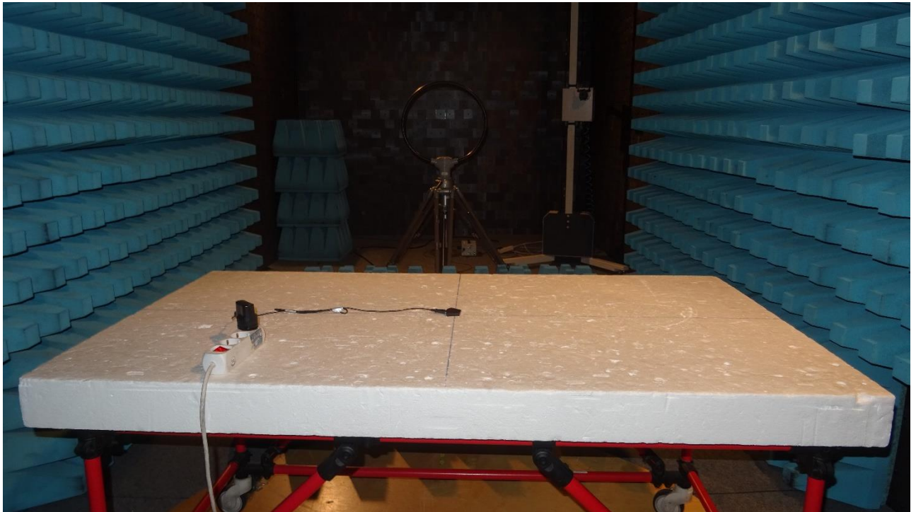
Picture 1: CDC, test setup radiated emission test 9 kHz - 30 MHz (front view), standby mode
