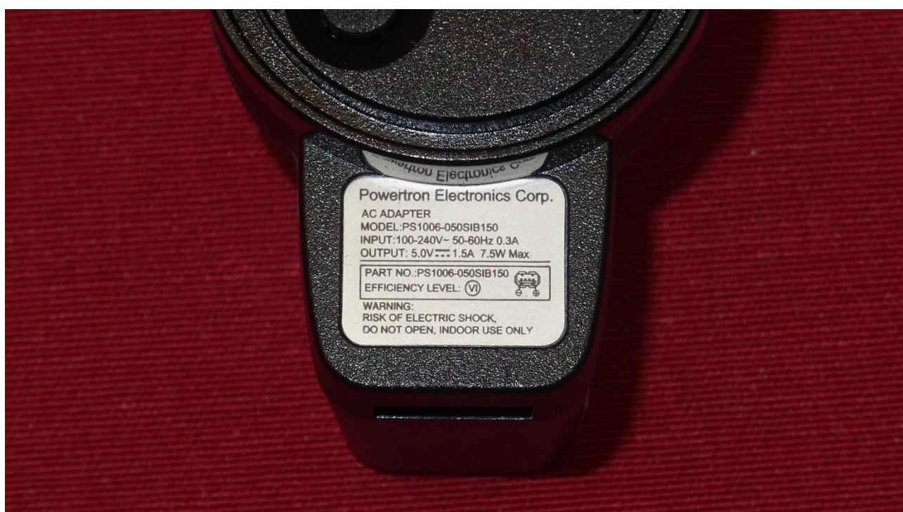
Picture 20: Name plate of power adapter
