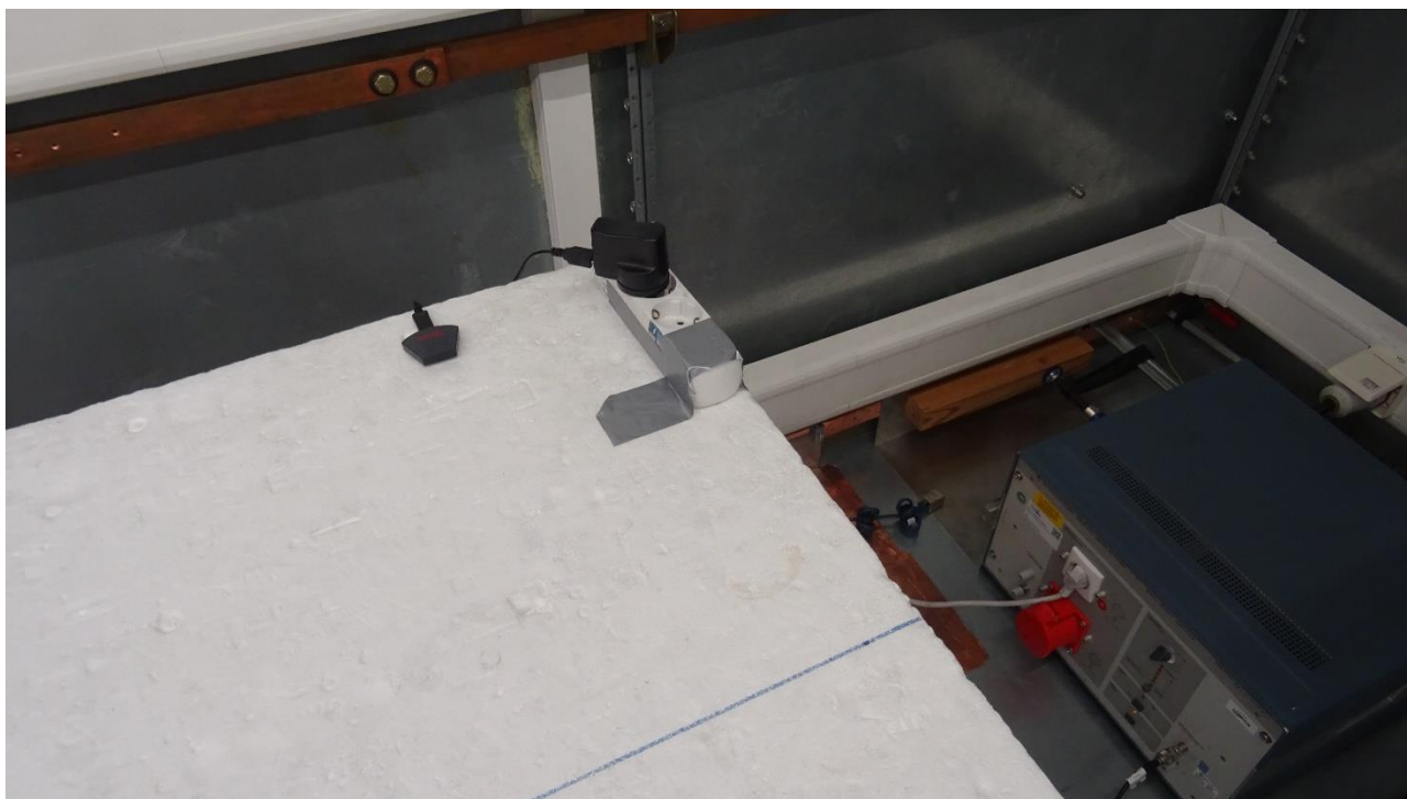
Picture 9: Test setup AC power line conducted emissions (front view), standby mode
