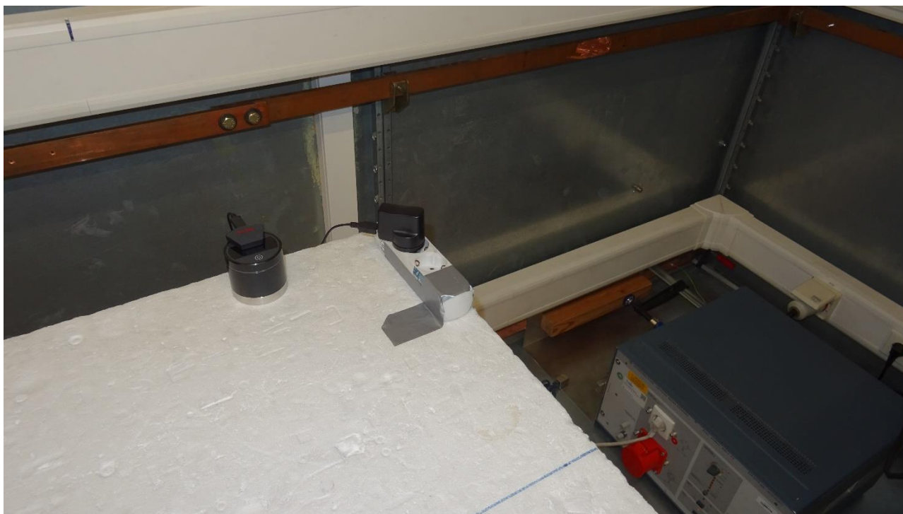
Picture 11: Test setup AC power line conducted emissions (front view), charging mode
