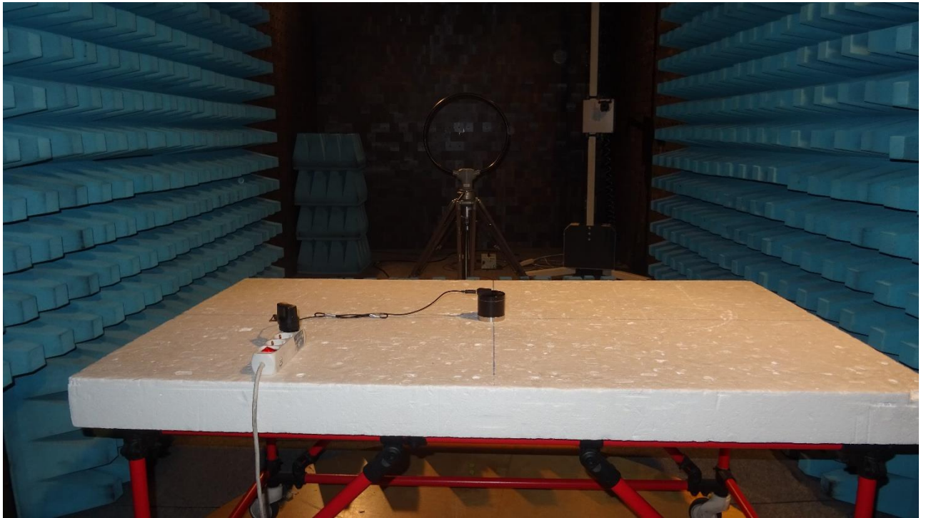
Picture 3: CDC, test setup radiated emission test 9 kHz - 30 MHz (front view), charging mode
