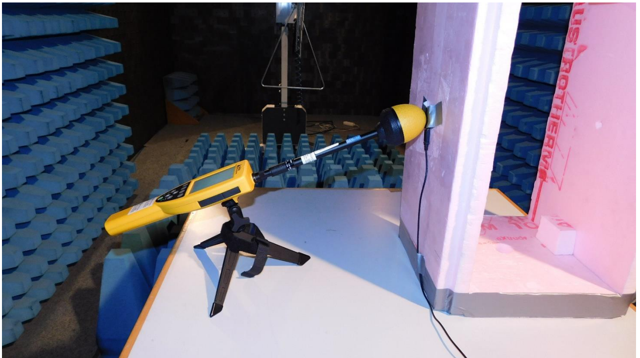
Picture 6: Position of maximum E-field emission measurement in standby mode
