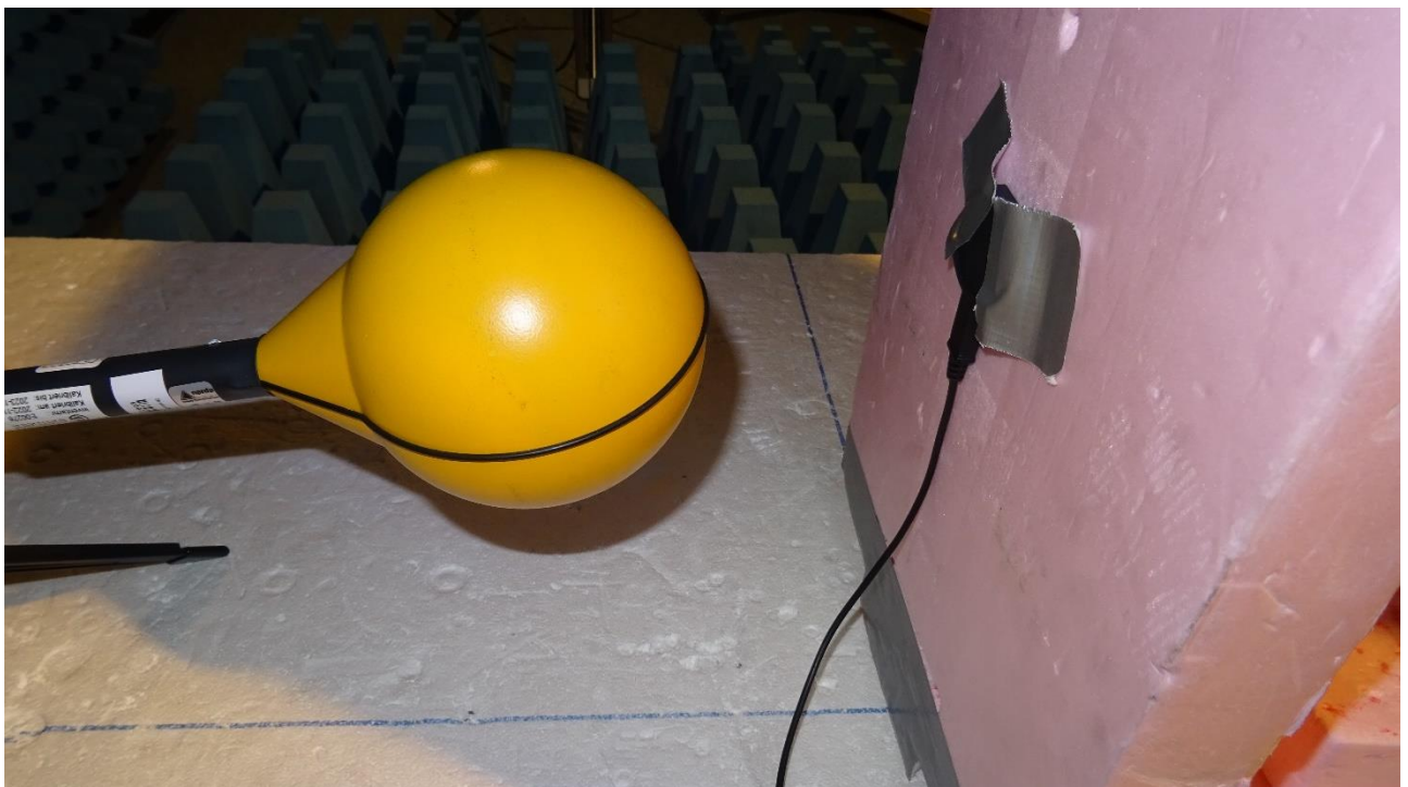
Picture 1: Setup of magnetic field test at a measurement distance of 15 cm in standby mode
