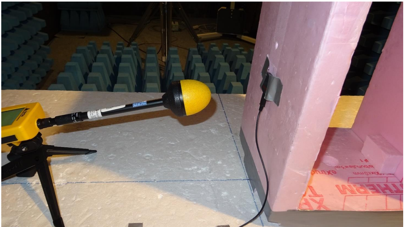
Picture 2: Setup of electric field test at a measurement distance of 15 cm in standby mode
