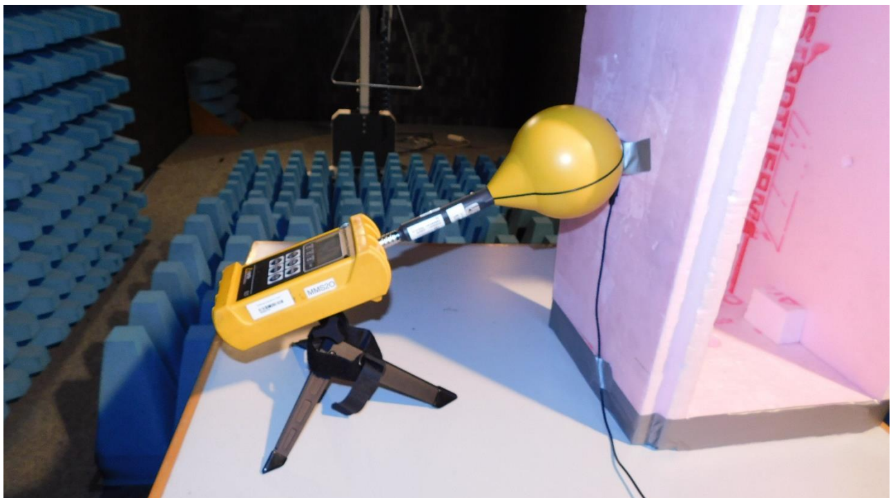
Picture 5: Position of maximum H-field emission measurement in standby mode
