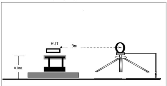
(B) Radiated Emission Test-Up Frequency 30MHz~1GHz
