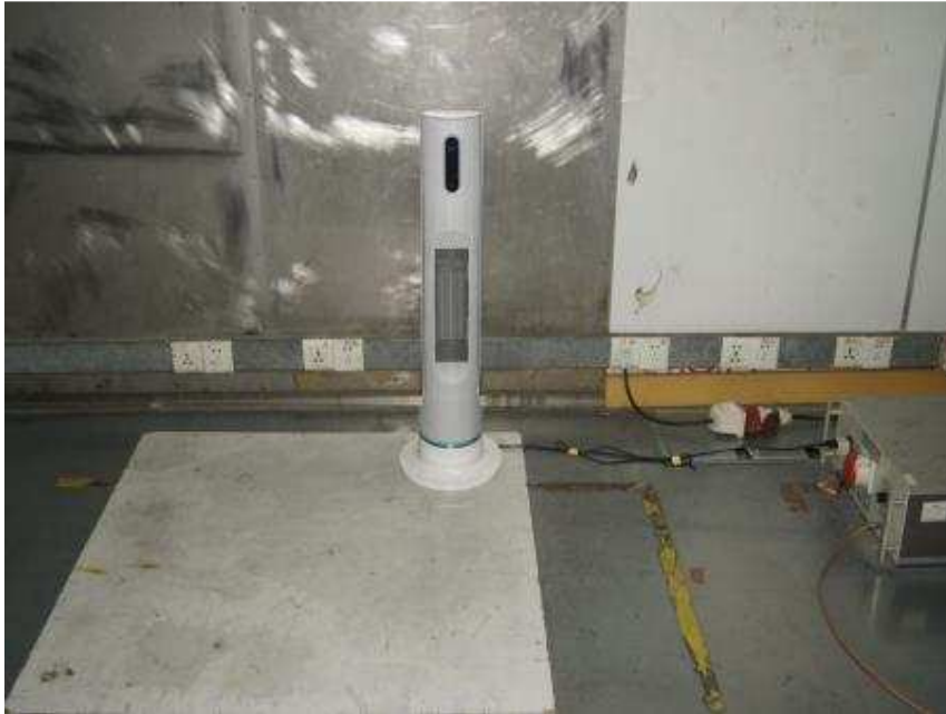
Photograph 6: Set-up for Radiated Emission, below 1GHz
