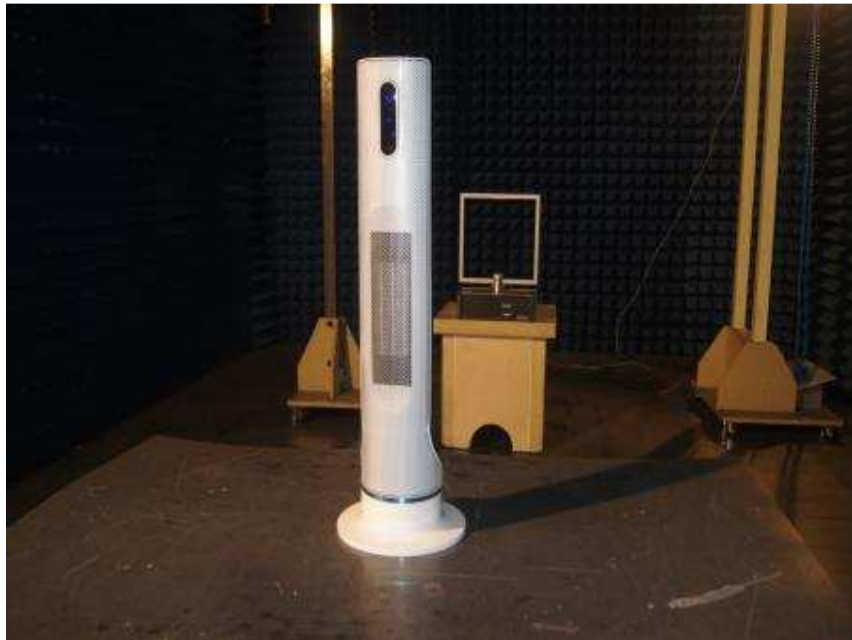
Photograph 2: Set-up for Radiated Spurious Emission (30MHz ~ 1GHz)
