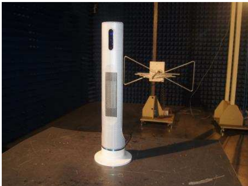
Photograph 2: Set-up for Radiated Spurious Emission (30MHz ~ 1GHz)
