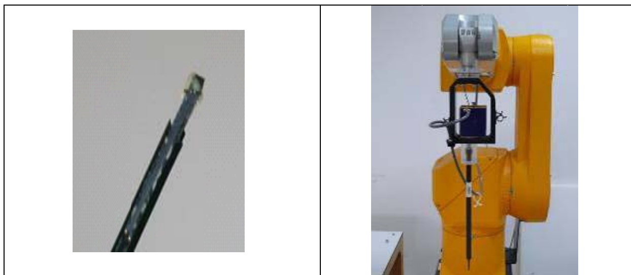
EX3DV4 E-field Probe
