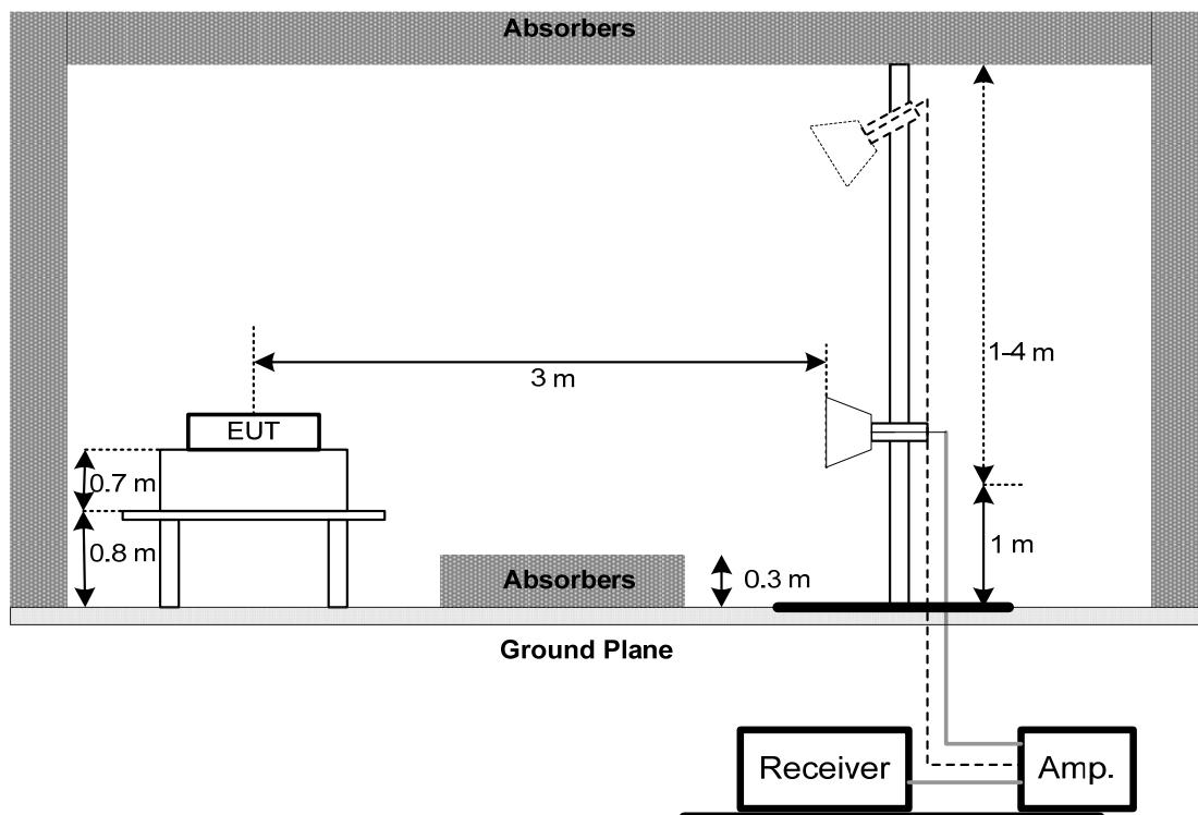
(C) For Radiated Emissions Below 30MHz
