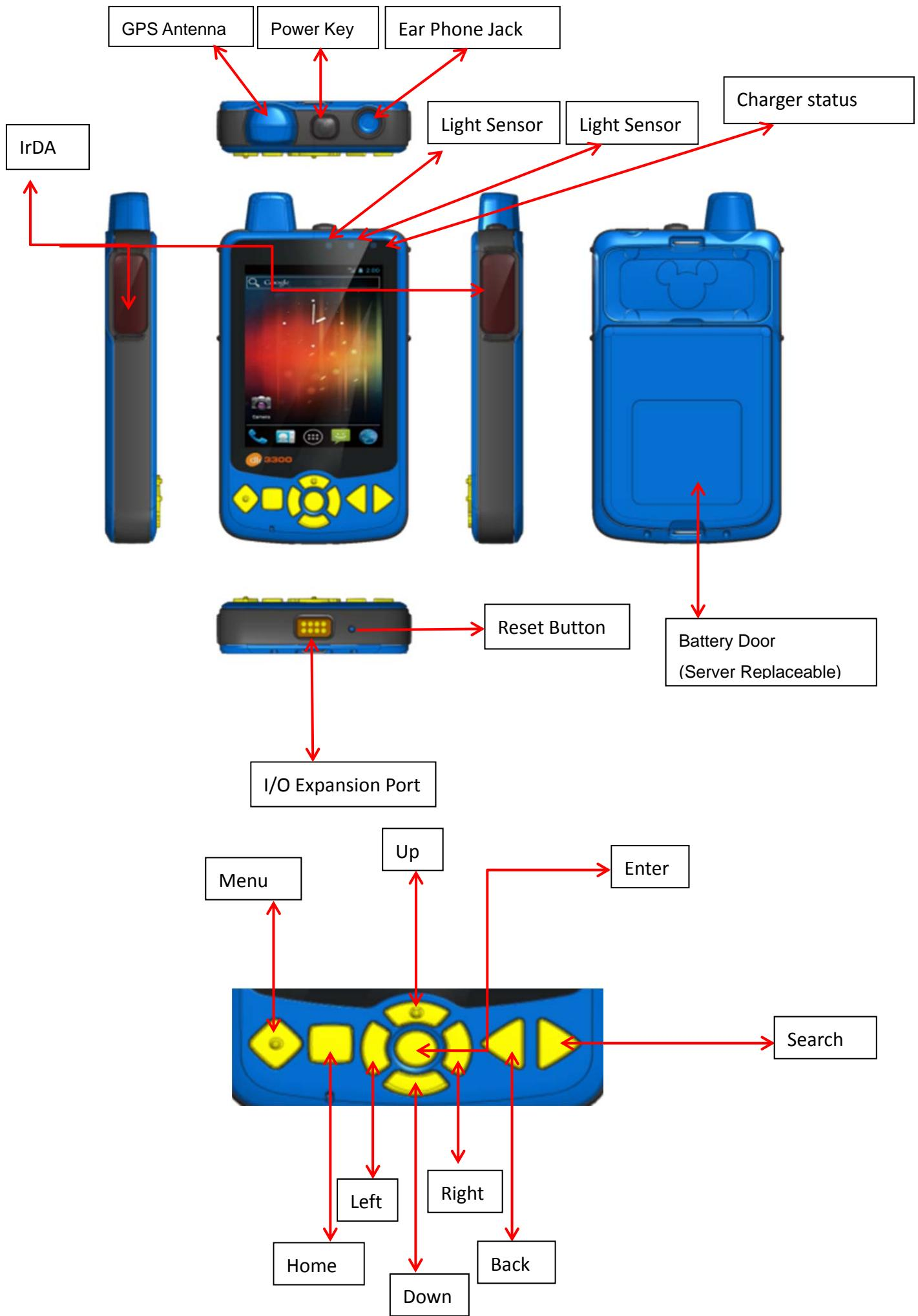
When the mobile computer is fully charged, press the Power key for three seconds to turn on the mobile computer. A locked screen will appear. Slide the lock button in either direction to unlock the screen
