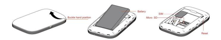
Tips: Always switch the device off and disconnect the charger before removing the battery.
