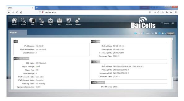
First part of the main display settings and network status information, such as IP address, SIM card status, type and quality of the network signal, whether it is roaming, with or without a new message, and traffic statistics, and system uptime, and so on.
