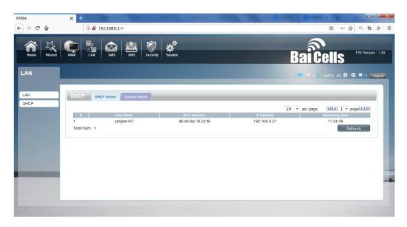
Leased Hosts: the R700 each wireless device list and USB device can view the Host name, MAC Address, IP Address, information about the Remaining Time.
