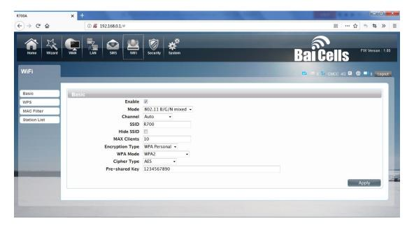
We can set the Wi-Fi configuration in this page, like B/G/N mode, Channel, SSID, WI-FI KEY and so on.
