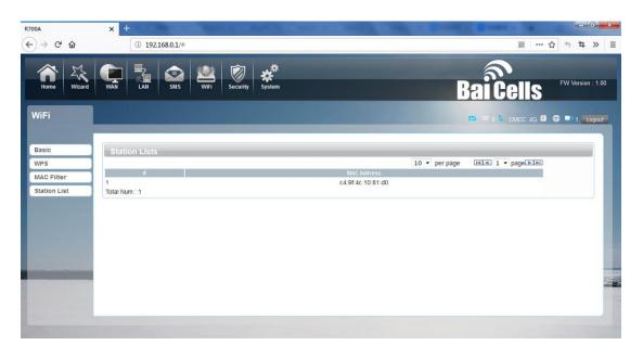
Show the information of wireless devices which are connected to the R700.
