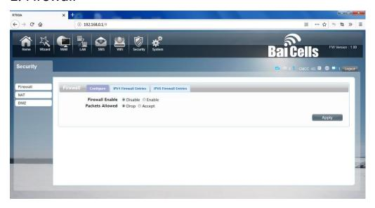
Firewall configuration: You can Disable or Enable the Firewall function. Also you can set the matching packets rule to receive or reject.
