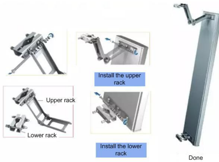
Figure 3-6 Assembling Procedure of Directional Antennas
