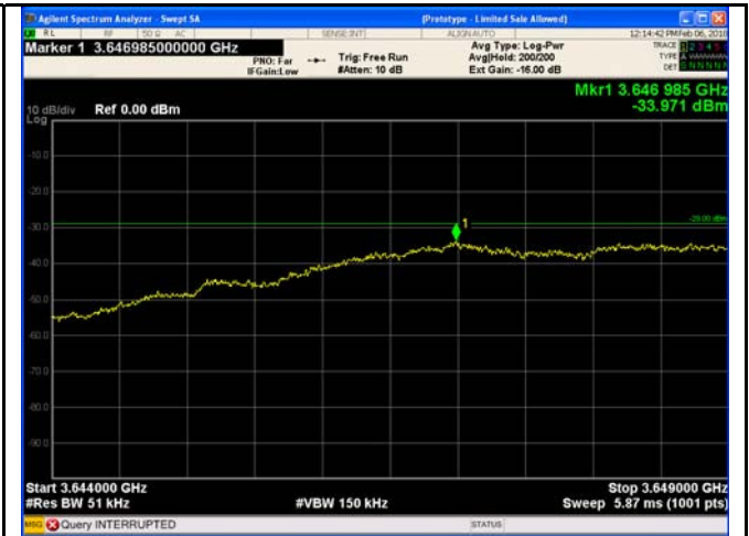
10MHz - 3644M-3649M Low CH 64QAM
