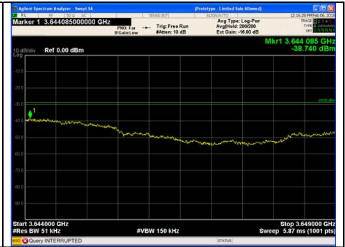
10MHz - 3644M-3649M Low CH 64QAM
