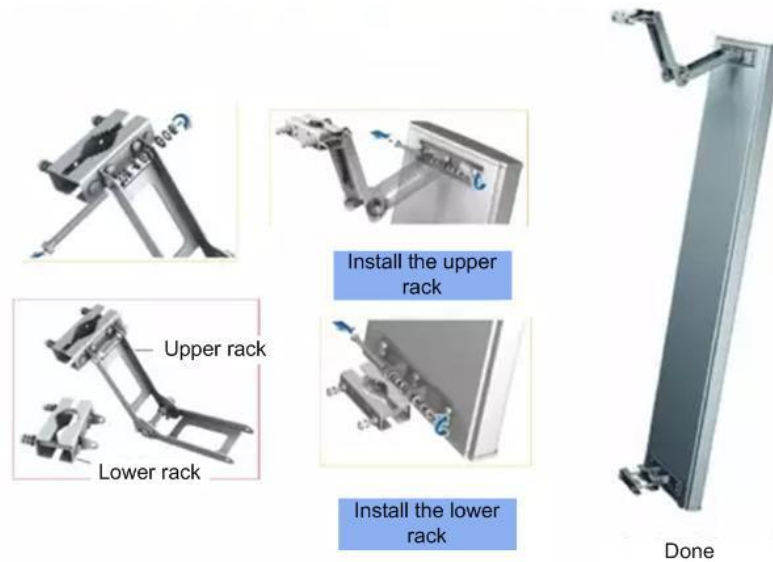
Figure 3-5 Assembling Procedure of Directional Antennas
