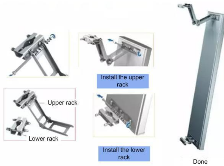
Figure 4-6 Assembling Procedure of Directional Antennas
