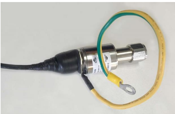
Figure 4-5 Weatherproof protection of the GPS RF Cable connection
