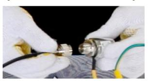
3. The connection point of RF cable needs to be weatherproofed. For more detail, refer to 3.5 Weatherproof Protection. After weatherproof protection, it is shown in Figure 4-5.
