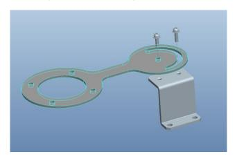
4. Fit the GPS antenna on the GPS mounting bracket 1 with an M4 screw. Vertical installation is required.
