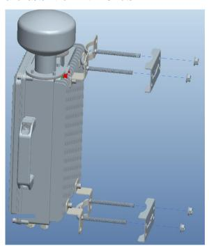
2. Hold the assembly up to the pole. Attach the two omegas to the threaded rods with M8 nuts.
