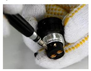
4. Insert the red power cable (48V) into terminal A, and insert the black power cable (0V) into terminal B, as shown in Figure 4-14.
