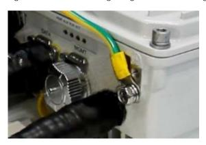
2. Unscrew another grounding screw, connect one end of the ground cable to the grounding screw of the device, as shown in Figure 4-18.
