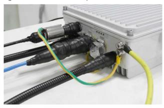
3. The other end of the ground cable needs to connect to a good ground (earth).
