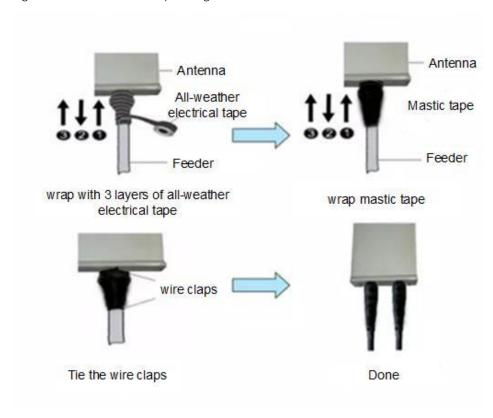
Be aware that at least three layers of tapes are needed, and make sure that the wrapping direction of the last layer is from the bottom up. The last layer should be tight enough to keep it from cracking.
