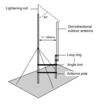
Figure 4-23 Omnidirectional Antenna Installation (2)
