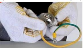
2. Connect one end of the GPS RF cable to the GPS lightning arrestor, as shown in Figure 4-4.
