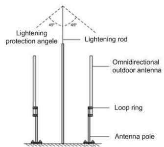
Figure 4-22 Omnidirectional Antenna Installation (1)
