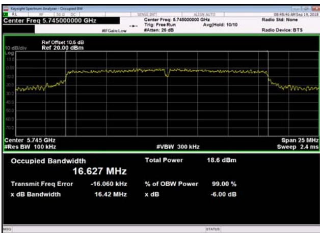
U-NII-3 6dB Bandwidth-802.11a(20MHz) ,5745MHz,Ant0
