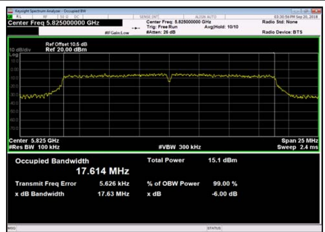
U-NII-3 6dB Bandwidth-802.11n(20MHz) ,5825MHz,Ant1
