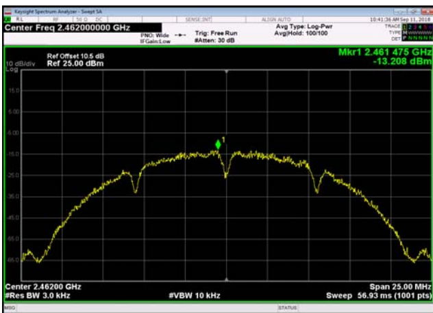
Power spectral density-802.11b ,2462MHz,Ant0
