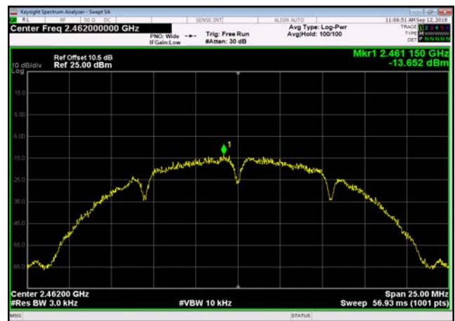
Power spectral density-802.11b ,2462MHz,Ant1
