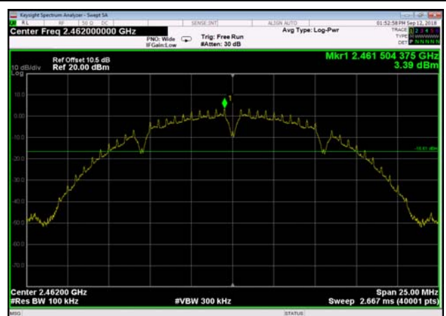
Reference Level-802.11b ,2462MHz,Ant1
