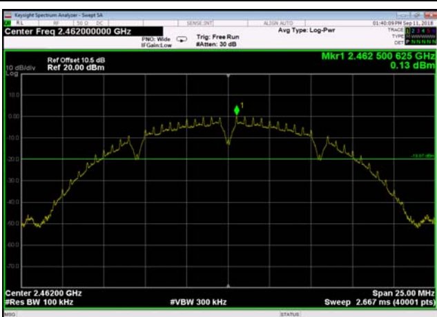
Reference Level-802.11b ,2462MHz,Ant0
