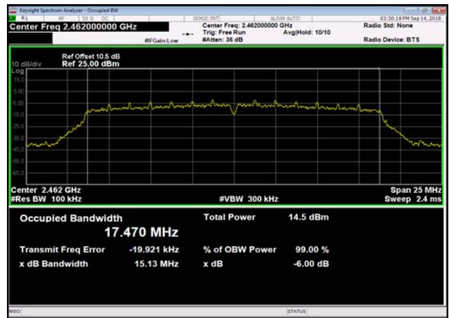
6dB Bandwidth-802.11n(HT20),2462MHz ,Ant1
