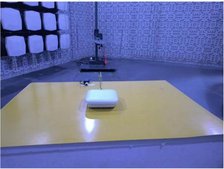
Unwanted Emissions that fall Outside of the Restricted Bands(Radiated) and Unwanted Emissions in the Restricted Bands (Radiated) above 1GHz
