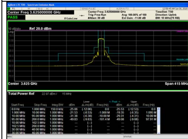
15MHz - Middle CH QPSK
