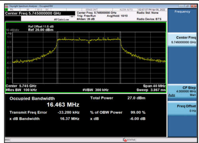
U-NII-3 6dB Bandwidth-802.11a(20MHz) ,5745MHz,Ant0
